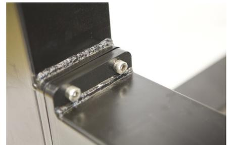
**\*As seen in the diagram above, the braces should be rotated correctly for the tool-box and shelf to sit at the correct height. Braces should be mounted so that the top and bottom are the larger flat surfaces\***
